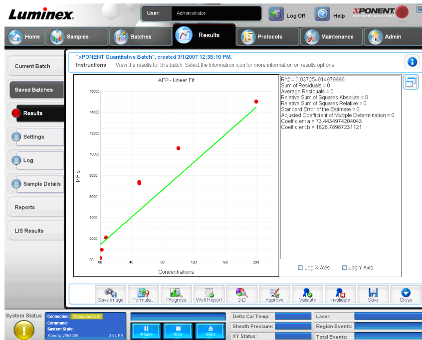
Figure A. Example of Linear Regression for the same immunoassay data as regressed in Figure B
