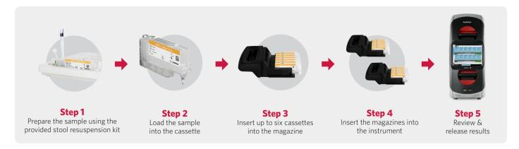
The operator prepares the sample, adds it to the scassette, puts the cassette in the magazine, loads the magazine into the ARIES® System, and the run will start automatically.
