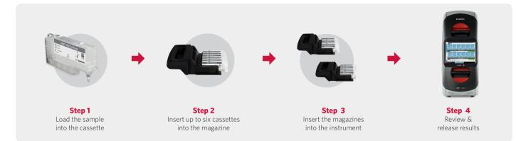
The operator simply adds sample to the sample chamber, puts the cassette in the magazine, loads the magazine into the ARIES<sup>®</sup> System, and the run will initiate on its own if the auto-run feature has been enabled.
