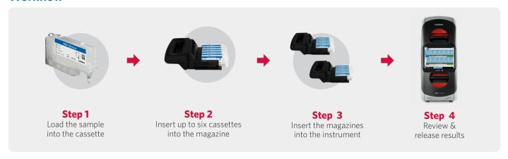
The operator simply adds specimen to the sample chamber, puts the cassette in the magazine, loads the magazine into the ARIES® System, and the run will initiate on its own if the auto-run feature has been enabled.
