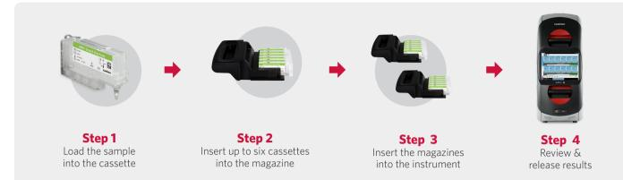
The operator prepares the sample, adds it to the cassette, puts the cassette in the magazine, loads the magazine into the ARIES<sup>®</sup> System, and the run will initiate on its own if the auto-run feature has been enabled.
