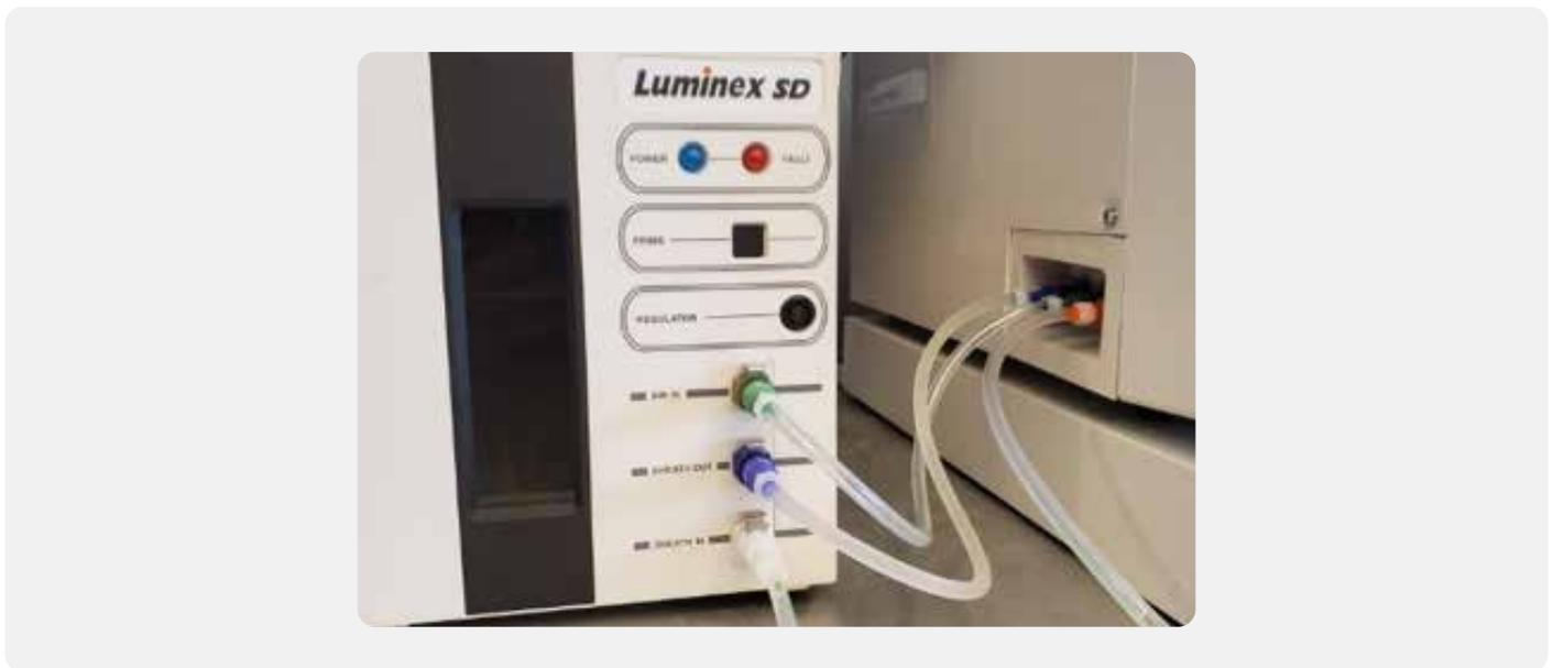
5. Run 6 Primes, 8 Backflushes, and 3 Washes to purge the old sheath from the fluidics lines within the analyzer.
