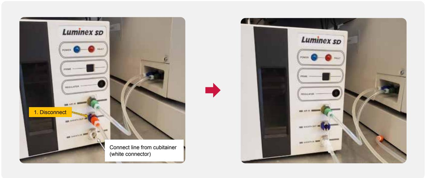
4. Once the SDS has finished filling, replace all tubing to standard positions (see **Figure 3**).
